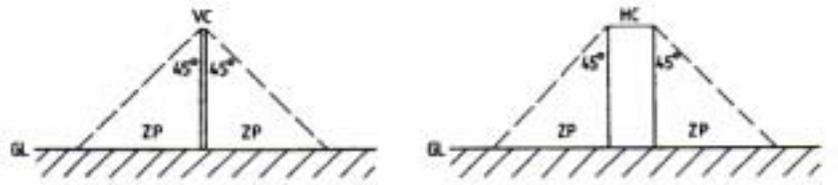
Plan view of zone of protection at ground level
