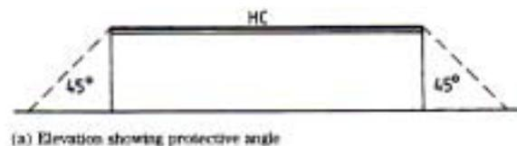
(a) Elevation showing protective angle
